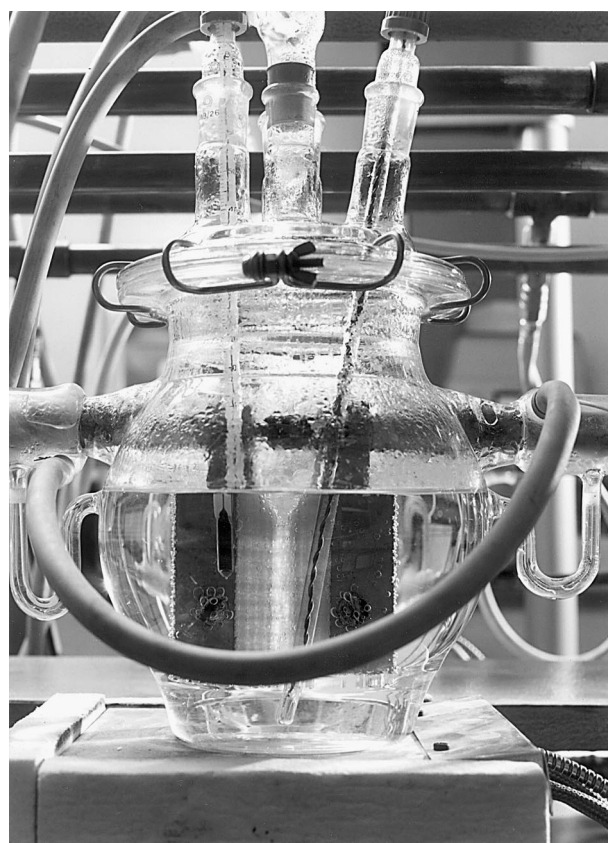
Figure 3 Measuring stress corrosion crack growth test at elevated temperatures.
